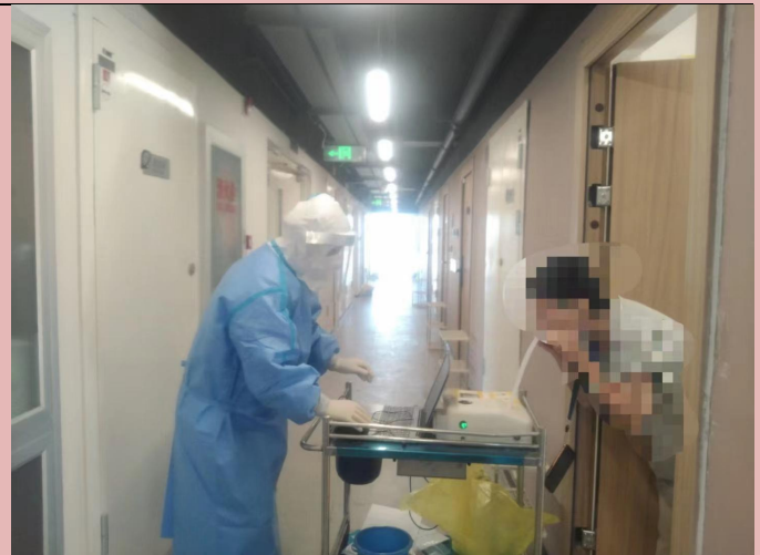
4. Exhaled breath condenser developed by our lab was tested with COVID-19 by Jiangsu Center for Disease Prevention & Control.
